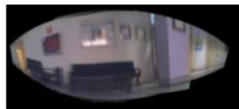
Fig. 20 Stitching of the image planes on the sphere.
