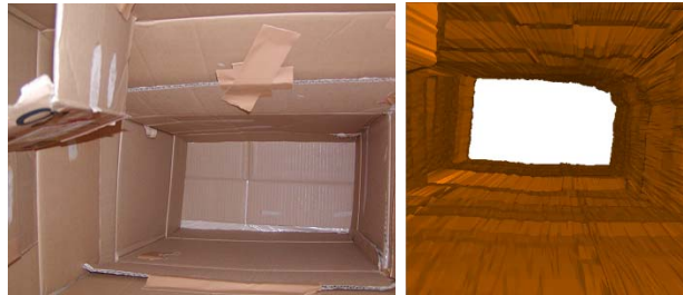
Fig. 22. Front view of the tunnel and constructed model
