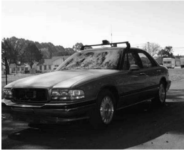
Fig. 1. LIDAR mounted on top of the vehicle.
